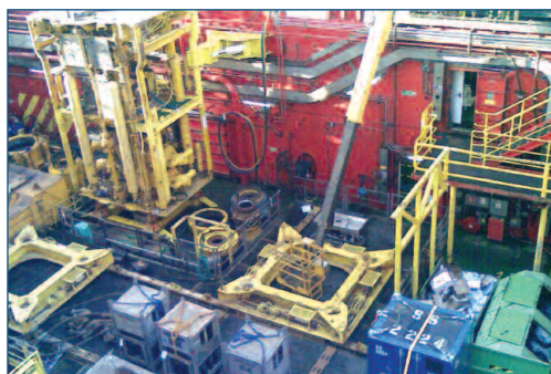
TREE SKIDDING SYSTEM & BOP GRIPPER ARMS, designed, fabricated and installed by Houder on the Stena Don.
