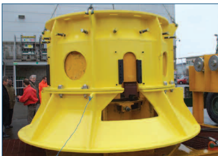
TREE SKIDDING SYSTEM & BOP GRIPPER ARMS, designed, fabricated and installed by Houder on the Stena Don.
